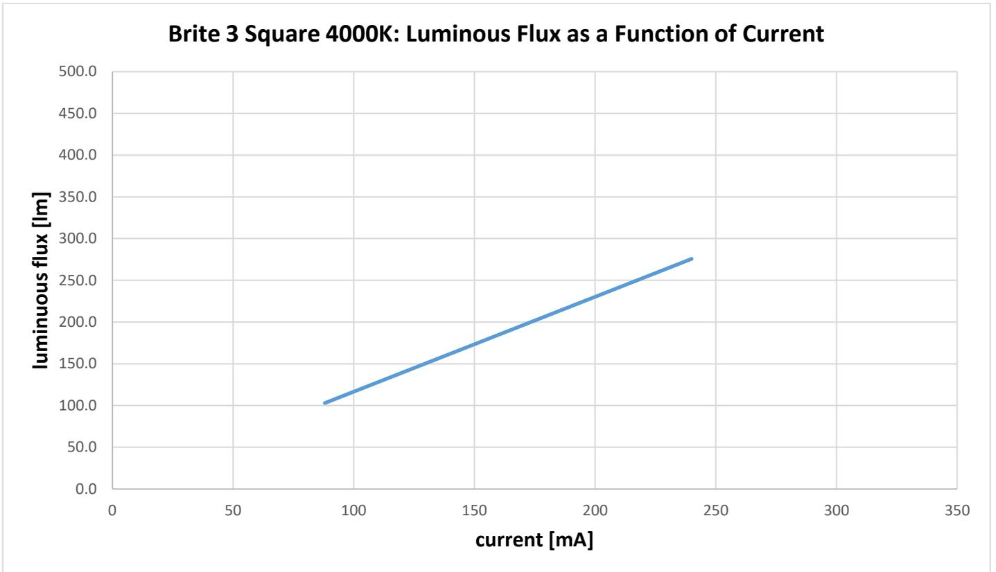
Figure 16: Luminous flux vs current, 4000K, level 1
