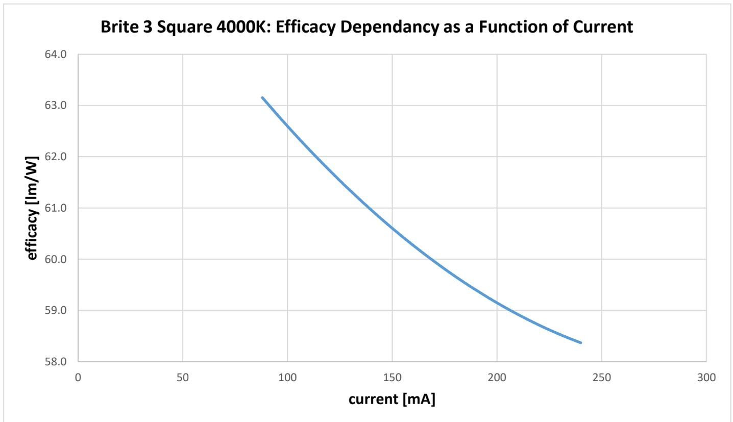
Figure 20: Efficacy versus current at room temperature, 4000K, level 1
