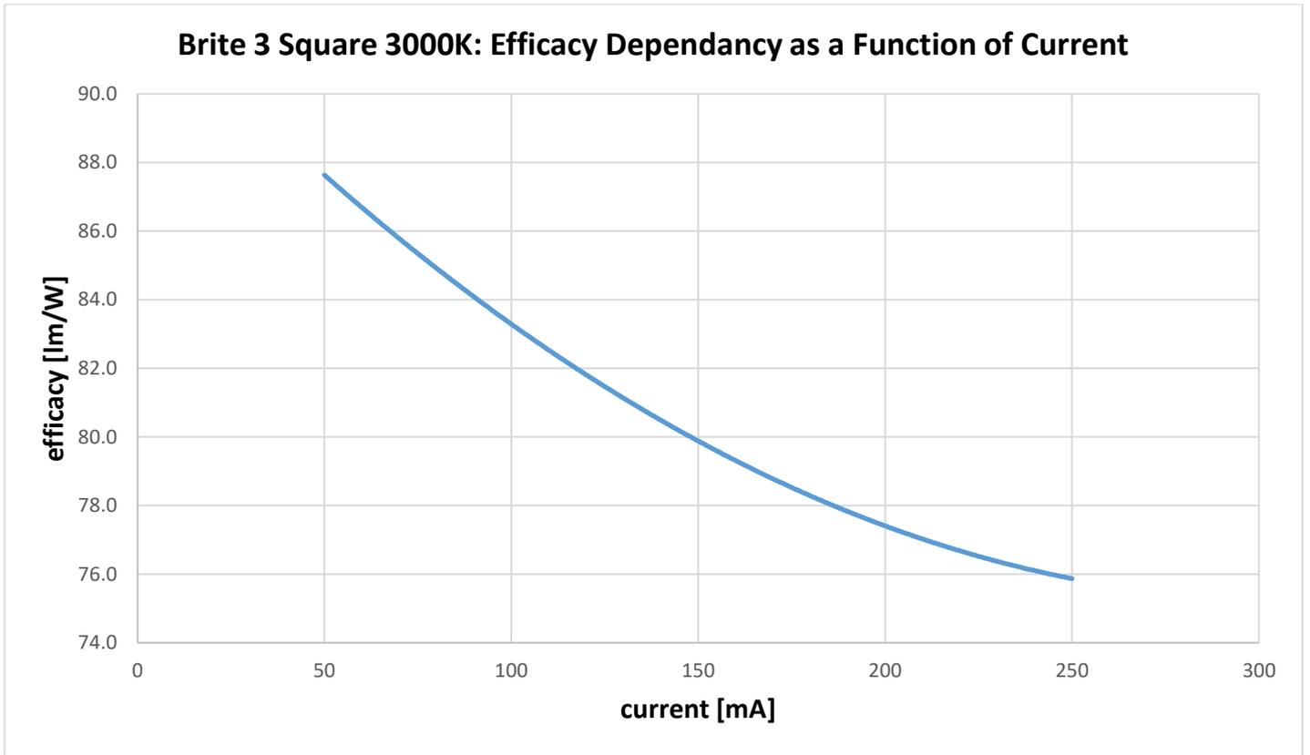
Figure 21: Efficacy versus current at room temperature, 3000K, level 1
