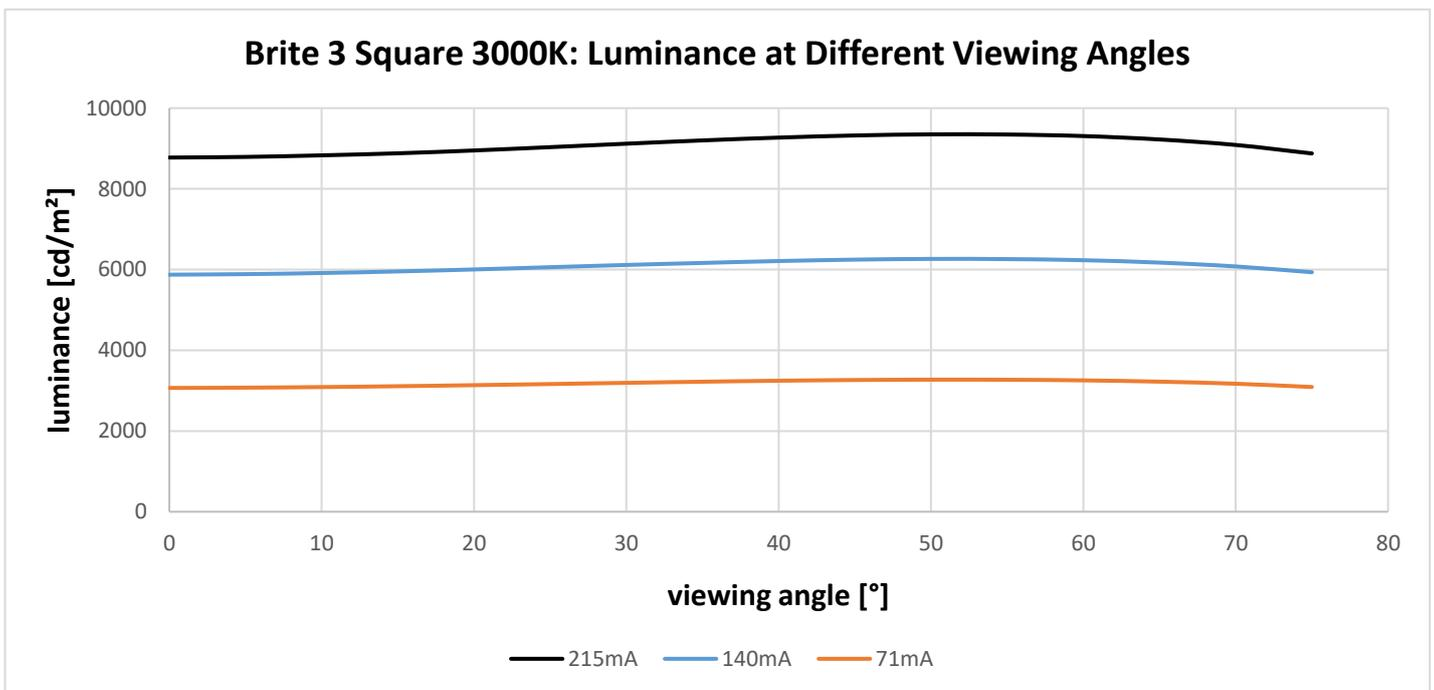
Figure 24: Luminance as function of the viewing angle. Driving currents  $I = 0.071 \text{ A}, 0.140 \text{ A}, 0.215 \text{ A}, 3000\text{K}$
