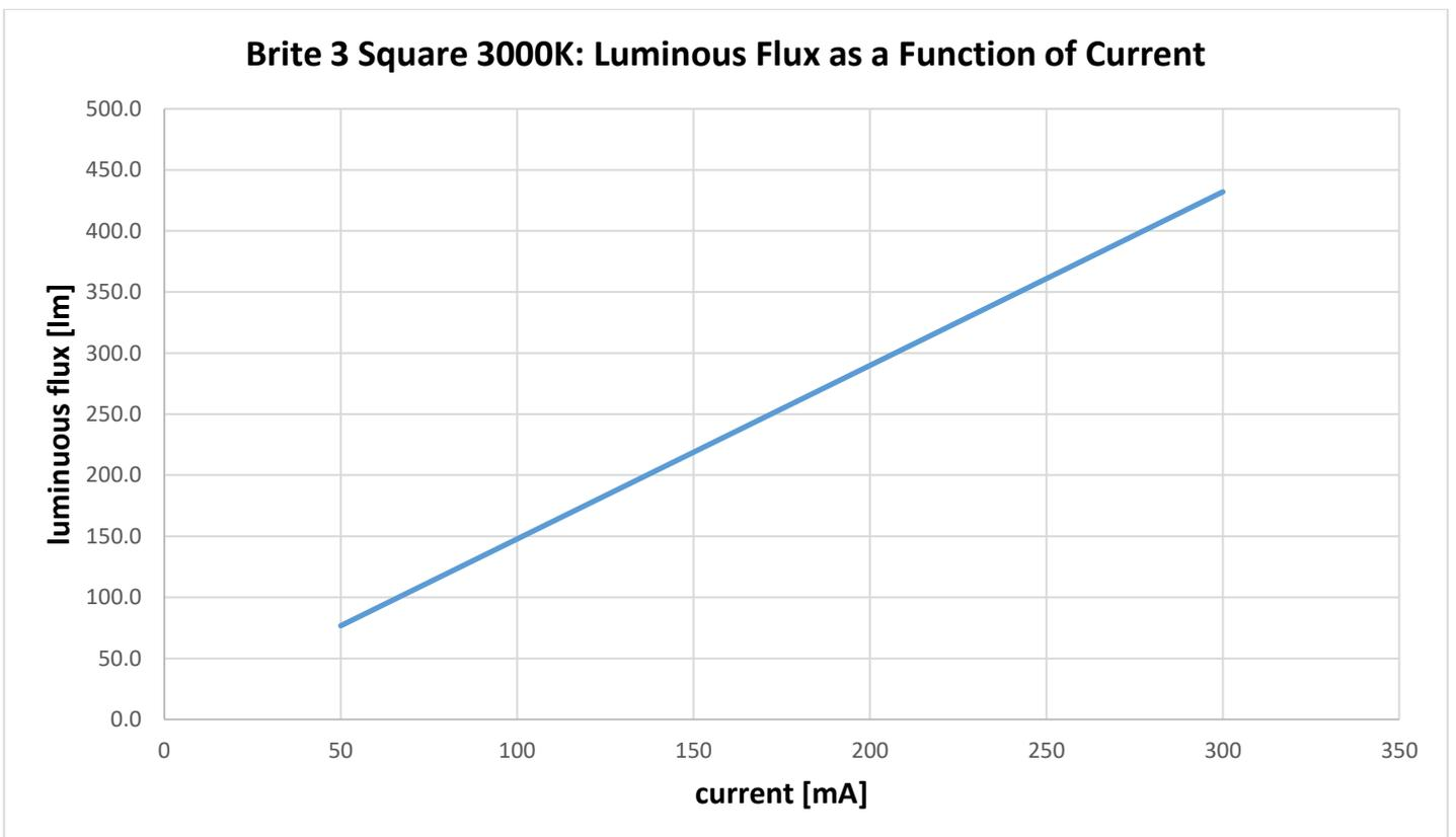
Figure 17: Luminous flux vs current, 3000K, level 1
