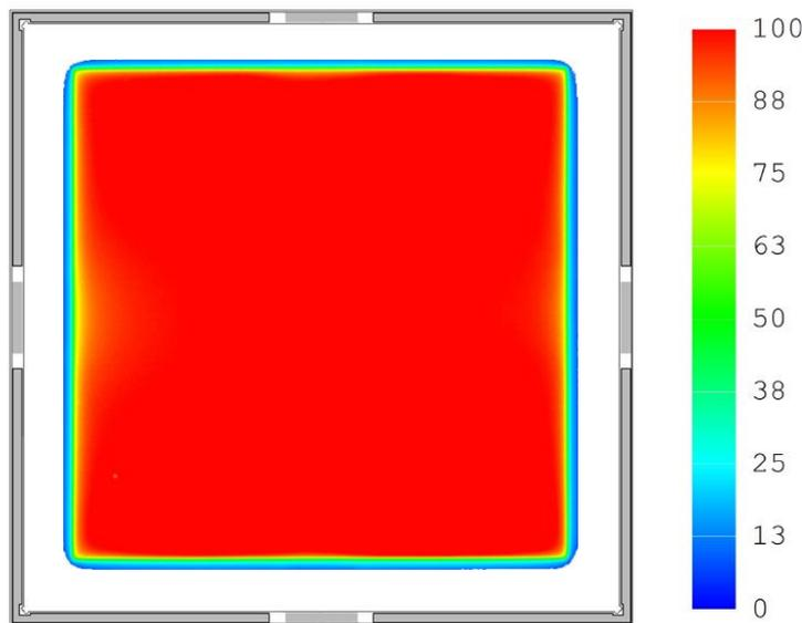
Figure 22: Typical luminance distribution for a Brite 3 Square Level 1. Operation conditions: vertical in air, RT (= 25 °C),  $I = I_{in\ rated}$
