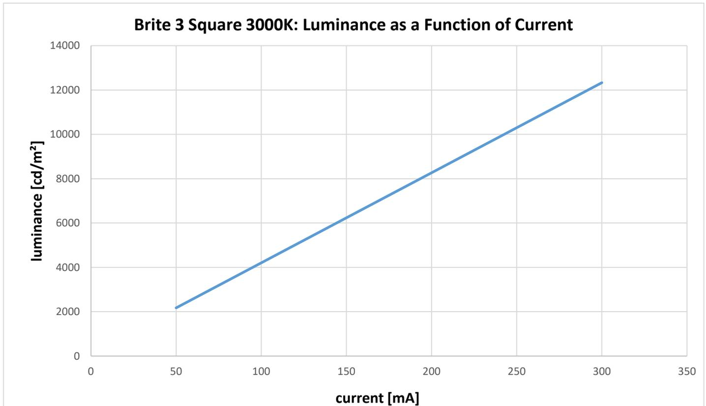
Figure 15: Luminance versus forward current at room temperature, Brite Square 3000K, level 1
