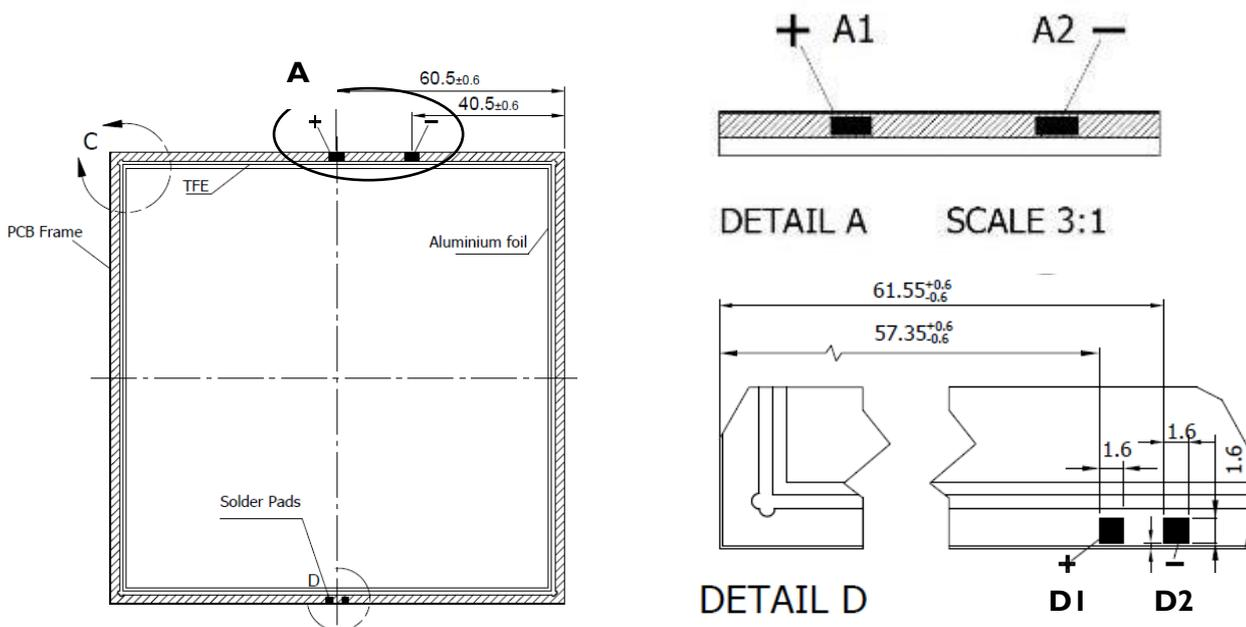
Figure 8: Contact pads of the Brite 3 Square Level 1
